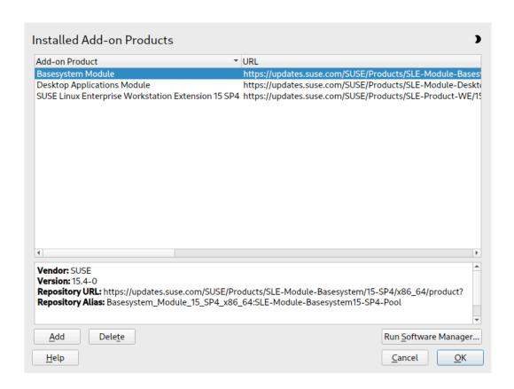
2. Choose the module or extension that should be removed and click *Delete*. Confirm the warning saying that all packages from the selected component will be removed.
